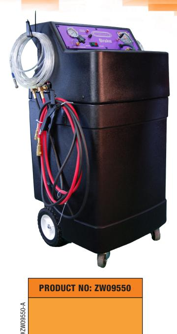
The Wynn's Brake Fluid Exchange machine provides a complete brake fluid exchange. It delivers brake fluid into the reservoir, simultaneously supplying vacuum to the bleed screws at all four wheels, ensuring a constant supply of new brake fluid and eliminating any air present or introducing new air into the system.
